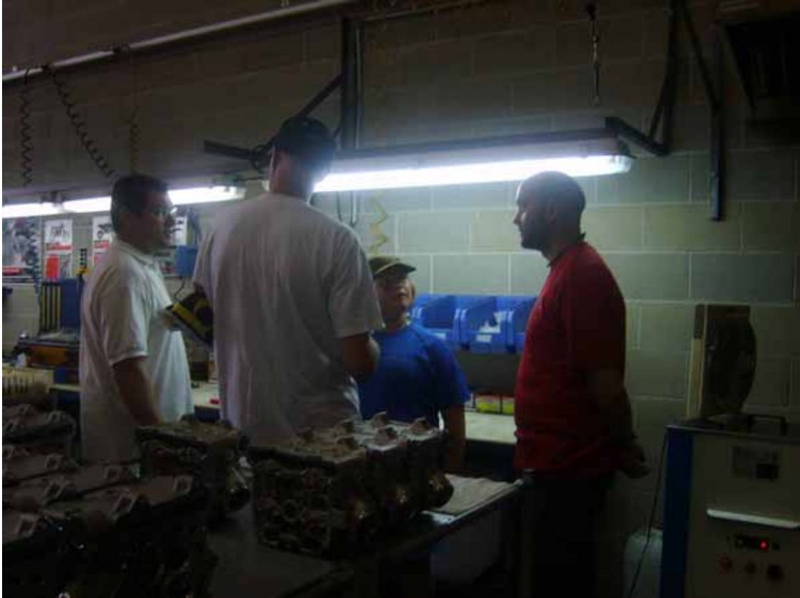
Figure 10. Discussion of the valve guide/valve seat assembly process. This is THE GUY who assembled your 4T heads. Furnace used to heat heads is visible in lower right of photo. Pneumatic hose to check for valve leakage is passing right behind Meredith's head (yellow line). Freezer used to cool guides and seats is not shown. Arbor press used to seat guides and seats is to the right of the furnace.
