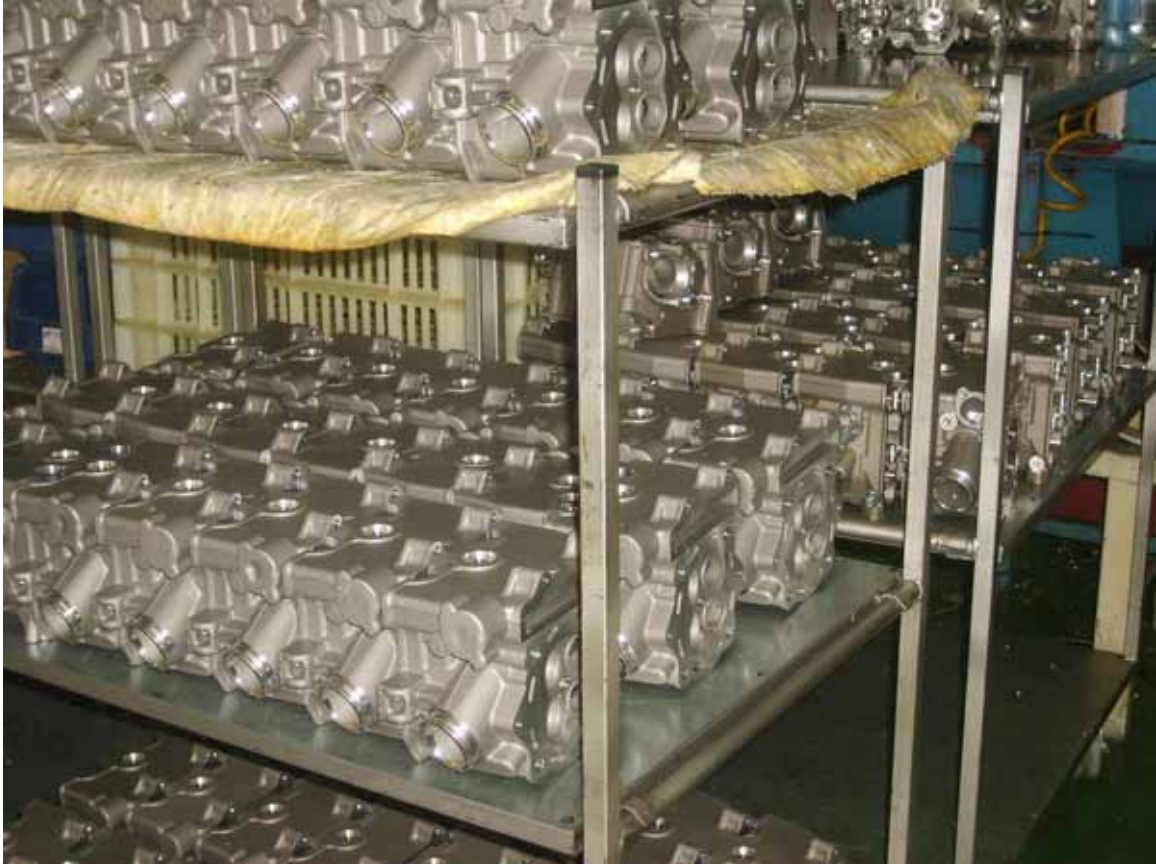
Figure 9. Cylinder heads after final machining but before valve seat and valve guide installation.
