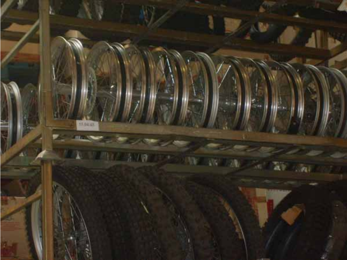
Figure 4. Wheel assemblies near the assembly line. Generally, wheels come laced with tires, sprockets, rim locks, and brake disks mounted. I am not sure of why tireless wheels are on the rack.
