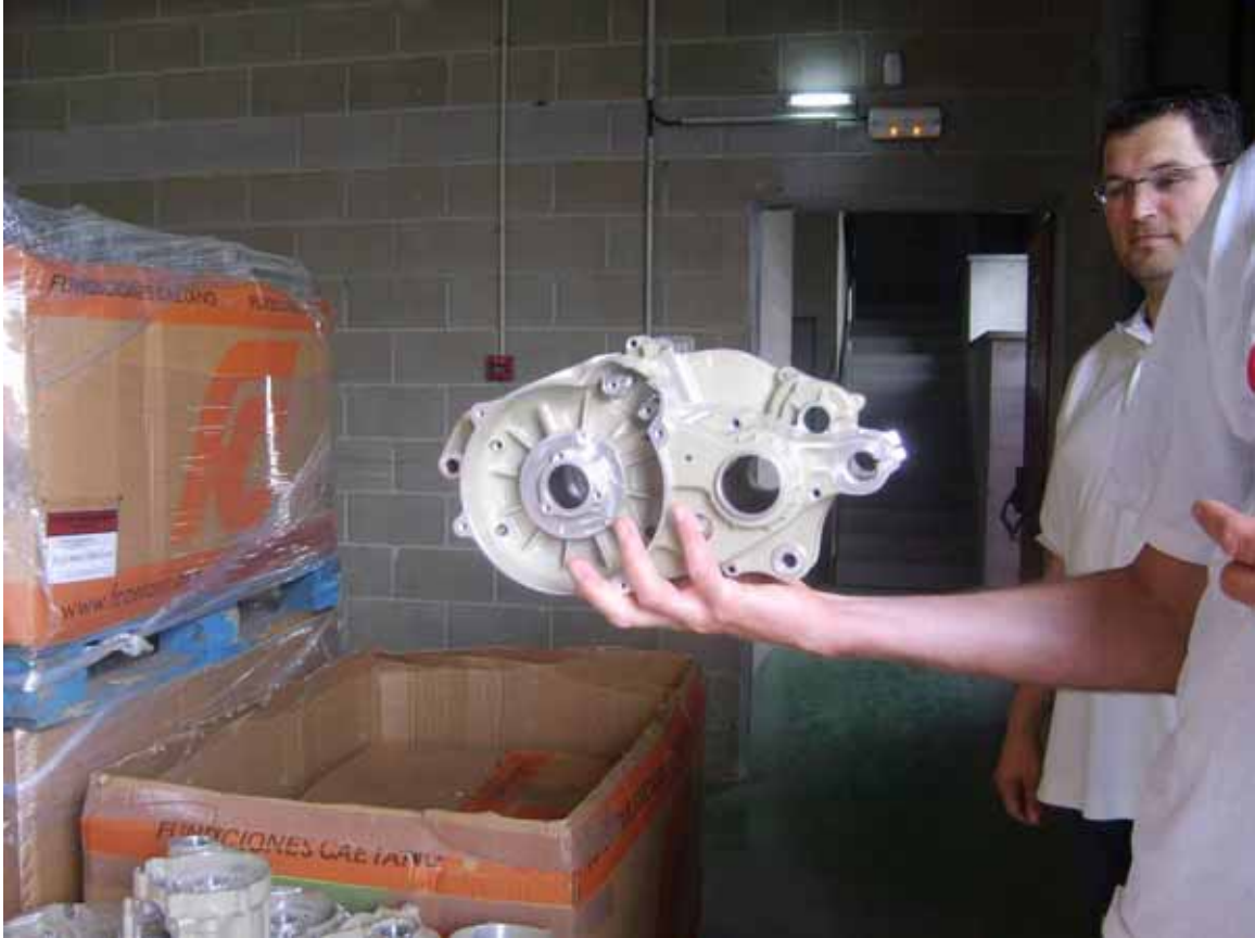
Figure 11. 2T magnesium engine cases. These things are INCREDIBLY light and trick. Really a nice piece of work. I was nervous about dropping them; Josep looks nervous, too.
