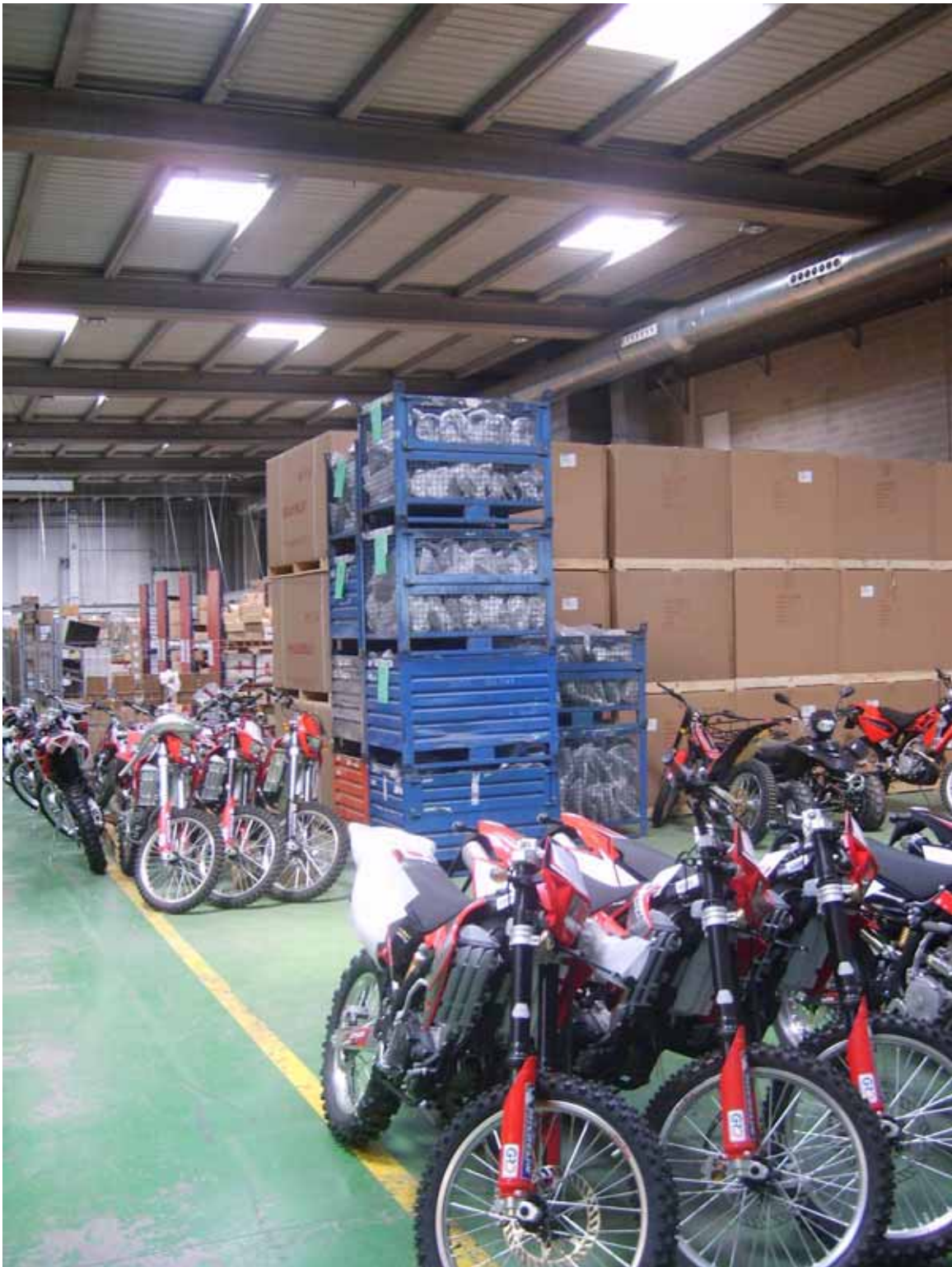
Figure 5. Foreground: assembled bikes ready for the US (note no 2T exhaust systems...FMF systems are installed in the US when the bikes arrive). Background: parts are in big blue crates. Further back in the photos are crates of PWK 38 Carbs, Marzocchi forks, etc. It's a gearhead's heaven.
