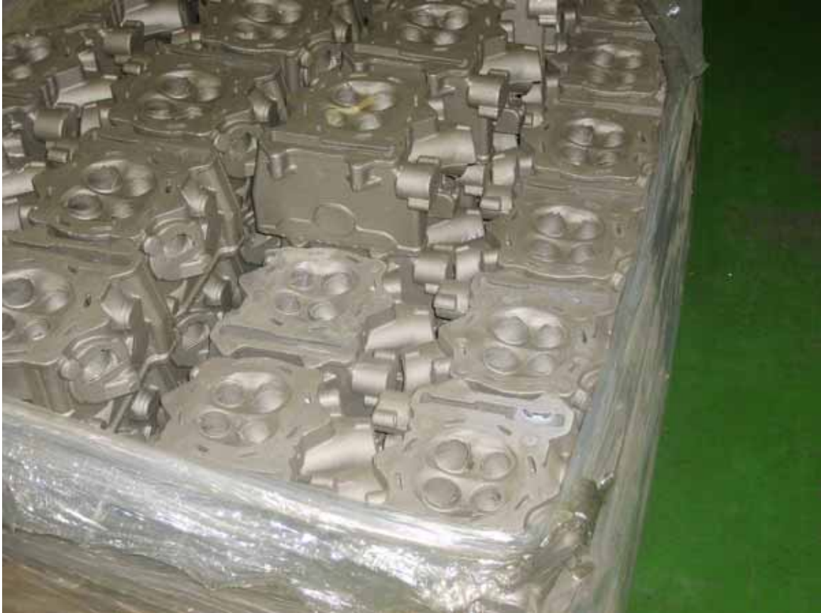
Figure 7. Raw 4T cylinder head castings, straight from the local foundry.
