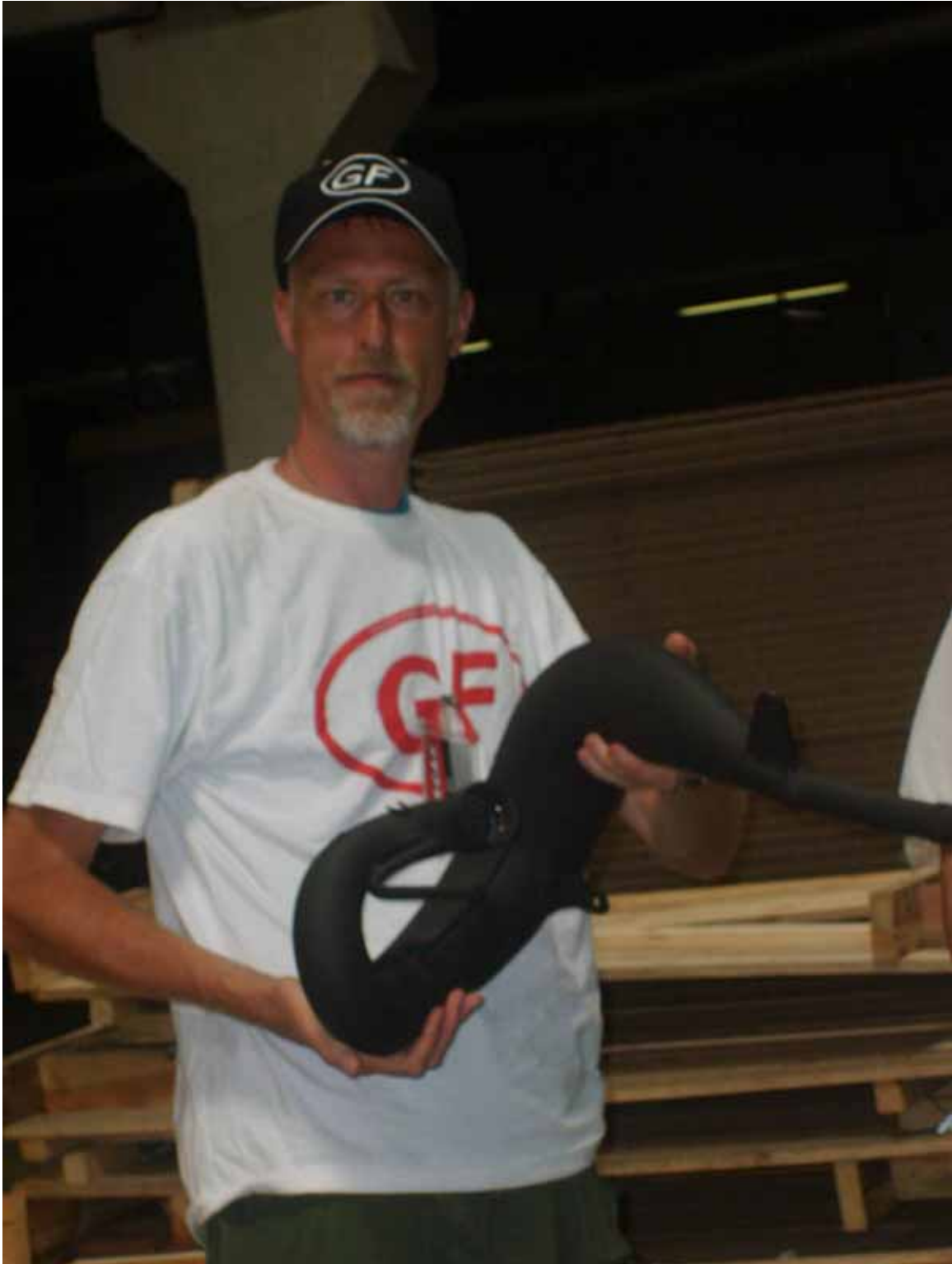
Figure 19. Author with Catalyst-equipped 2T exhaust. Really heavy. The catalyst is the “traditional” honeycomb configuration. Weight might be due to dual layers for noise abatement and structural rigidity (rock damaged exhaust may crush honeycomb, restricting gas flow).
