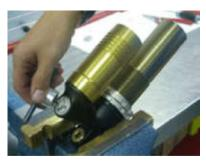
Proceed as follows (J.8-J.9): unscrew the ring nut with a suitable wrench, extract the parts paying attention to the dismantling sequence in order to correctly effect then the reassembly.
