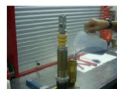
P repare the diaphragm with assembled 0 R (we advise using a new one for each replacement). F ill up the reservoir with oil and insert the diaphragm into the reservoir, (see photo).
