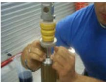
K eep the fork rod in position and run the fork rod guide to fit the shock absorber tube.
