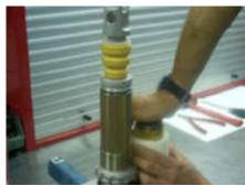
P roceed by topping up until reaching approx. 2 cms (0.8 in.) from the body edge. Then, execute 4 or 5 alternating strokes of 5 - 6 cms (2-2.4 in.) to bleed the air left under the piston unit.
