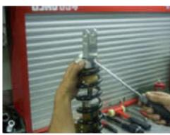
Measure the free length of the spring. USEFUL LIMIT: 9.59-9.70 in. When the spring length is lower than the useful limit, replace the spring.
