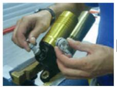
A fter having completed the check, insert again the piston, the disk, the spring and the ring with slots. R emove the cone holding shaft from the plug, screw the ring and insert it in the slot applying a light pressure. Lock the assembly with the plug at a torque of 30 Nm (3 kgm; 29.2 ft/lbs).
