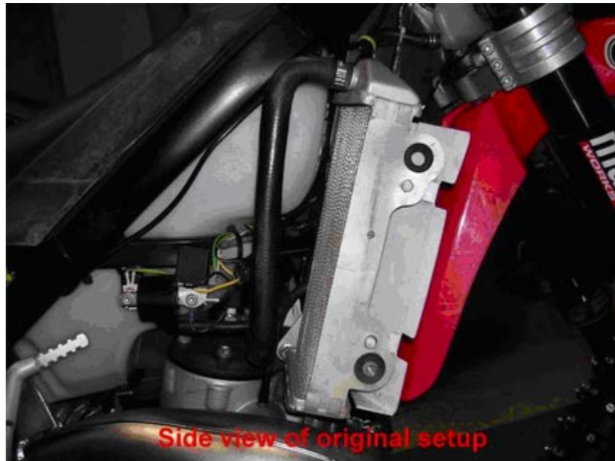
View of radiators (after removing shrouds)
