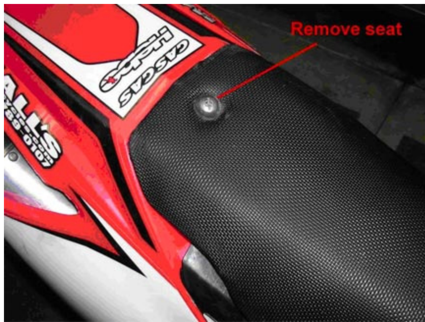
Remove seat (using Phillips screw driver)
