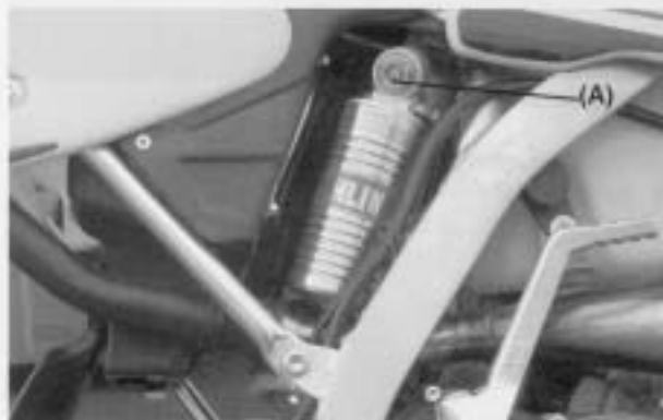
(A). Compression dampening adjuster.
