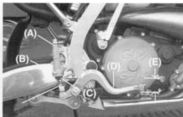
(A). Master Cylinder (B). Piston (C). Push rod (D). Rear Brake pedal (E). Lock nut
