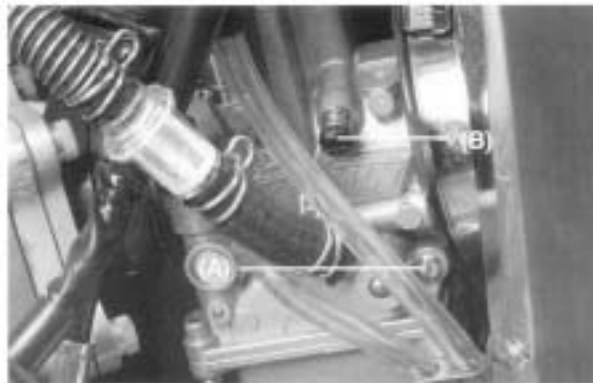
(A). Air mixture screw (B). Idle speed adjustment screw.
