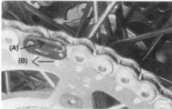
(A). Clip (B). Direction of Chain Rotation
