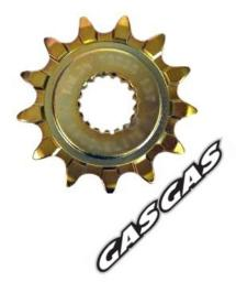
All Talon gearbox sprockets are manufactured 'in-house' in the UK. Available in our standard design only, these front sprockets are made from case hardened chromoly-steel, zinc coated and heat treated for long life.
